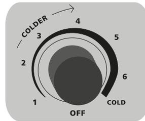
Conversely, if the ambient temperature is very low, or the cooler is empty or lightly loaded, the interior temperature might drop below 0°C. This could cause the evaporator to freeze. To avoid this, adjust the thermostat slightly to the left.
